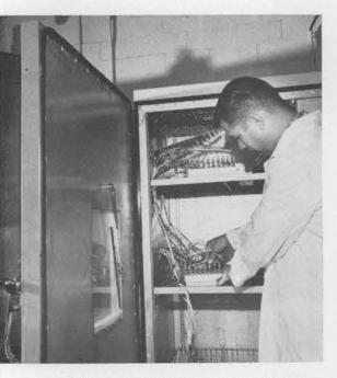
ROQUE FELICIANO (4632-2) is preparing a set up for testing the resistance of resistors to moisture. Humidity can be varied from fine spray to a "soak" test as some design difficulties are only found under full moisture conditions. Resistors may be tested while in the humidity chamber or before and after immersion.
